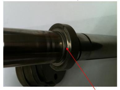
This is where the sealant ends up lubricates thrust plate. Grease / Vaseline could be put here during reassembly to prevent start up squeaking.
