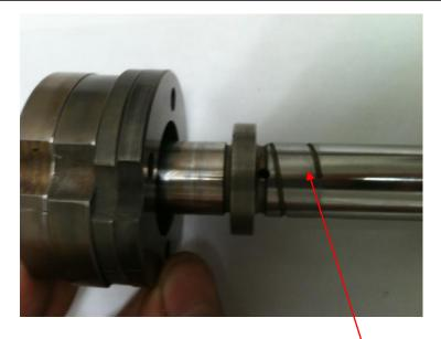
Sealant will work around the gear in this area
