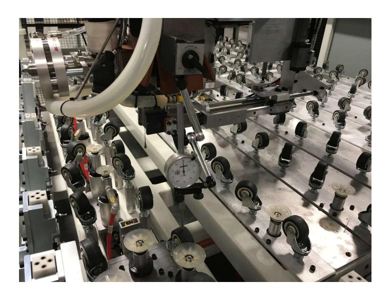
Push the head around to each roller position and adjust height as needed
