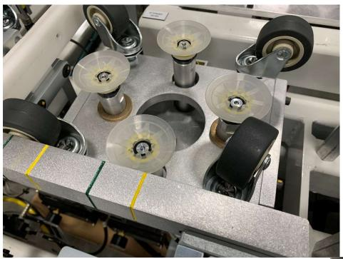
When extended the cleats on the cup should contact the bottom of the glass once the lips flatten out
