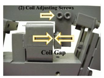
NOTE: This inline drive unit may be equipped with a coil containing a **thermal overload protection** device (identified by the letter "T" following the catalog number on the coil ID plate). If the coil becomes too hot, due to an 'out-of-adjustment' condition, it will shut down, and remain in this state until an optimum operating temperature is achieved.
