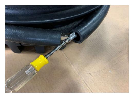
Once started with a nut driver you could use a power drill with a long <u>fixed</u> extension to complete the closure of the band clamp
