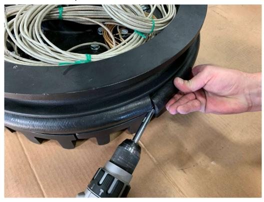
Once tightened you will see the end gap has closed leaving approximately a 1/8 gap which will close up once inserted into a drum
