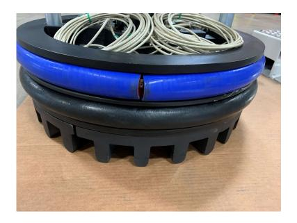
The upper ring seal used is made of a softer durometer material and will haver a larger end gap but it to will close up once inserted in a drum
