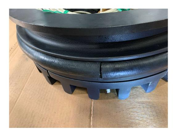
End gaps should be offset 180deg form each other (it doesn't matter which is facing to the front or back)
