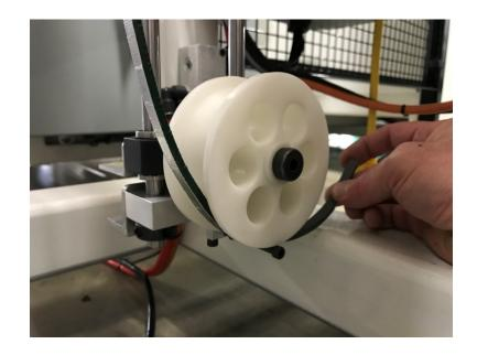
Make sure to feed spacer **between** roller and guide
