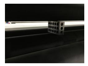
If the front and back indicators do not read the same and you have verified parallel of the rollers with your gage blocks, adjust the jamb bolt on which ever side is off to correct readings
