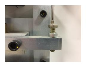
If the front and back indicators are reading within .005 and there is a gap between your gage block and the roller on one side you can adjust that side by loosening the slave shaft coupler and adjusting each side independently from the other to correct gapping issue.
