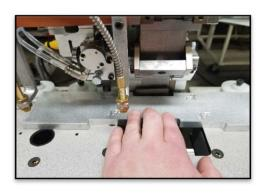
Center the Calibration plate over the nozzle, verifying the depth probe is also in a pocket cutout. The IG DEPTH should match the depth of the cutout on the CALIBRATION plate +- .010 . Flip the plate around to test the depth probe at different depths.
